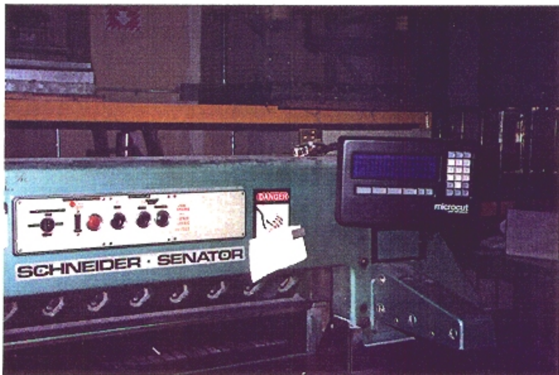
Typical display mounting. Display can be mounted anywhere on the front of the cutter, but is generally placed to the right side high enough to avoid interfering with the operator.
