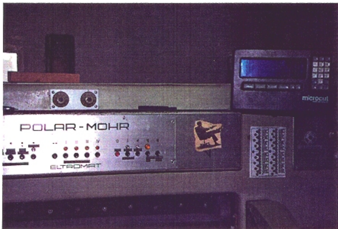
Typical display mounting. Display can be mounted anywhere on the front of the cutter, but is generally placed to the right side high enough to avoid interfering with the operator.
